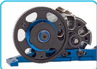
New one-piece motor mount
