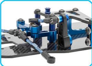
Updated dual bellcrank steering system and floating servo mount
